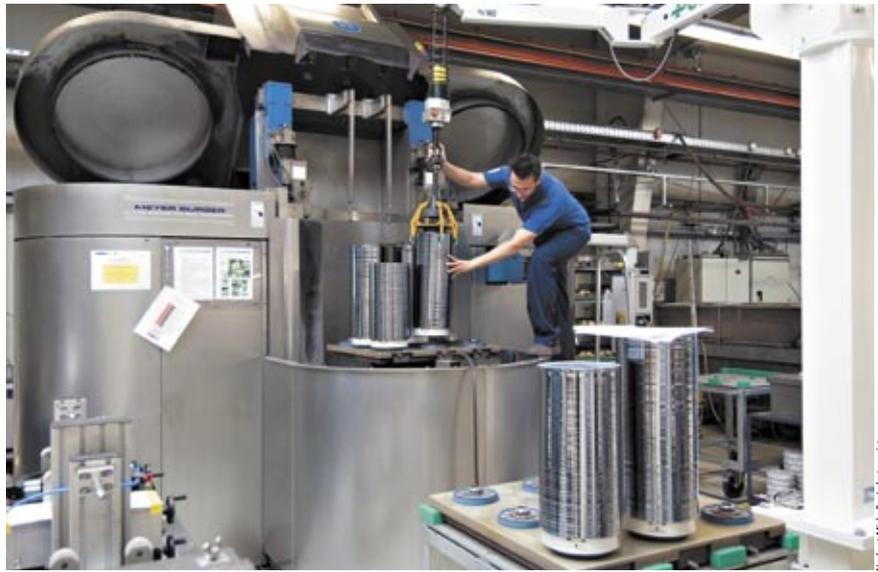
**Hard and harder:** During the sawing process you can tell the difference between high- and low-ohmic silicon ingots at this point – high-ohmic silicon is harder.
