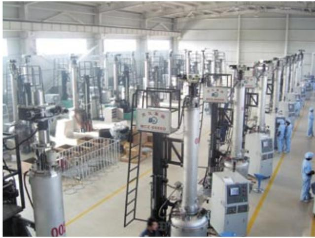
The production halls at Xi'an Longi in the Chinese province of Shaanxi: The company obtains wafers with very low oxygen content using the Magnetic Czochralski process.
